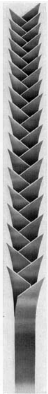
Looking down the cutting edge of a cross-cutting Hand saw—as it appears in an enlarged view.
