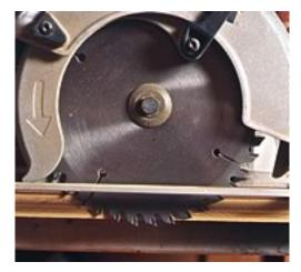
Don't worry about what's below. Set the depth of cut so that a full tooth of the blade extends below the workpiece. You'll be cutting right into the surface of the sacrificial table.
