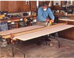
To load a sheet of plywood, tip the table onto a pair of scrap wood spacers. Lift the ply onto the spacers, and lift the ply and the table together.
