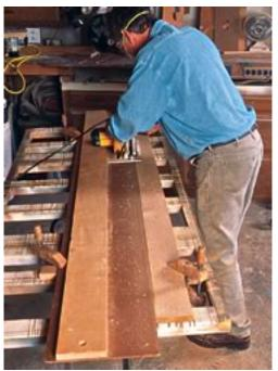
You can use the long guide to put a straight edge on a waney board. Block up the guide so that the workpiece just fits under it. Then nudge the waney edge of the workpiece under the guide's base. Clamp both guide and workpiece, and rip off the edge.
