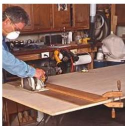
The short, straight guide is used for intermediate rips and long crosscuts.
