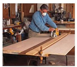
The long, straight guide makes quick work of ripping a full sheet of plywood. When the cut has been made, the halves of the sheet stay put, supported by the cutting table.
