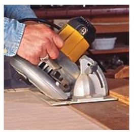
To make mitered edges, assemble a guide with its base cut to 45°. Align the angled layout line with the mitered edge of the base.
