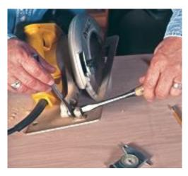
Use a dial indicator to check that the blade is parallel to the edge of the saw base (left). Adjust the base to correct any error (right).
